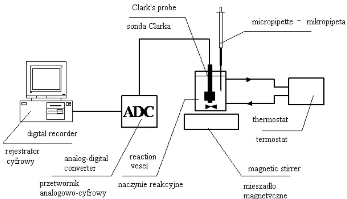
Fig. 1. Diagram of the measuring system to be tested mitochondrial respiratory activity
